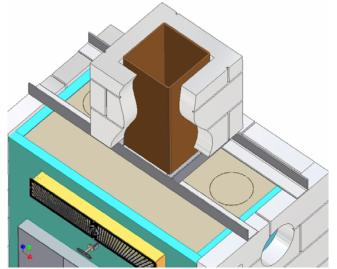
FIGURE 7B: MASONRY CHIMNEY INSTALLATION
